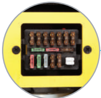
CONCENTRATED FUSE BOX FOR EASY INSPECTION
