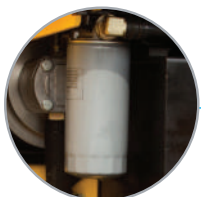
HYDRAULIC RETURN OIL FILTER IS EASILY ACCESSIBLE
